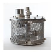
The Rotorflush RF200R is a coarse screened self-cleaning strainer that connects to the suction hose of surface mounted pumps. The RF200R is fitted with a single sheet of perforated stainless steel mesh which forms the filter cage. Standard perforated mesh sizes are 3mm and 6mm. The RF200R filters have a capacity of up to 220 litres per minute. All our filters have an internal cleaning rotor that is water powered by taking a 'T' off the output of your pump
