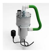
The RF200A-E and RF200R-E are self-cleaning intake filters for attachment to the suction hose of surface mounted pumps. These filters are the same as the RF200A filters and RF200R strainers with one difference. Unlike the 200A and 200R filters the backwash is not powered by the pump they are attached to - they have their own integral backwash pump to keep the filter mesh clear. This allows you to vary the output of your pump without affecting the
