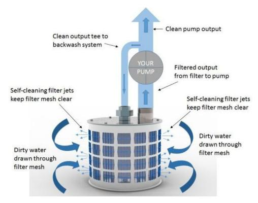
200AS self-cleaning intake filters provide protection against blokage for surface mounted pumps and other connected equipment. These are stainless steel dirty water suction intake filters with a capacity of up to 220 litres / minute.
