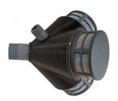
The RF100 Triplex trebles the capacity of the RF100 self-cleaning filter to a maximum usable flow (of 90 litres per minute. The RF100 Triplex self-cleaning inlet filter comprises three self-cleaning filter heads which keep the filter mesh clear, preventing the filter from blocking, protecting the pump and other equipment. It is easily installed to your pump's suction pipe and is robust and reliable. The filter can be used for many domestic and light
