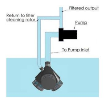
The filter uses a proportion of the pump's output to supply a feed to the internal backwashing rotor. The twin jets of the cleaning rotor rotate at about 60 rpm in each filter head, cleaning their whole screen every ½ second. Approximately 20-30% of the pump output is required to supply the cleaning rotor.
