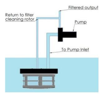
The filter uses a proportion of the pump's output to supply a feed to the internal backwashing rotor. The twin jets of the cleaning rotor rotate at about 60 rpm, cleaning the whole screen every ½ second. Approximately 20-30% of the pump output is required to supply the cleaning rotor.
