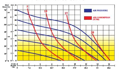
AIR PRESSURE: Tested at 690 kPa (not to exceed 861 kPa)
