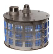
The RF400AR self-cleaning filter is for use on the suction side of surface mounted pumps. The RF400AR is an extremely tough stainless steel basket filter that protects pumps and other connected equipment form blocking and blinding. It can be fitted with tough nylon filter mesh or stainless steel screens and can filter from 60 microns to 6mm. The RF400AR can handle up to 1000 litres per minute. The patented self-cleaning mechanism in the filter
